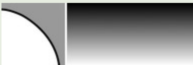
Cavetto moulding and resulting shadow pattern
